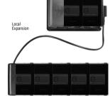
The maximum number of Uni-I/O $^{\text{TM}}$  Wide modules that can be connected to a single CPU controller is limited. For details, please refer to the specification sheets of the UniStream $^{\text{TM}}$  CPU or any of the relevant Local Expansion Kits.
