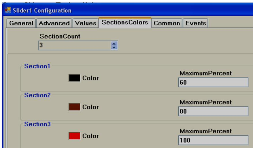
**Sections colours:** It is configured bands for the sections to show different colours for Labels and Ticks in Slider.
