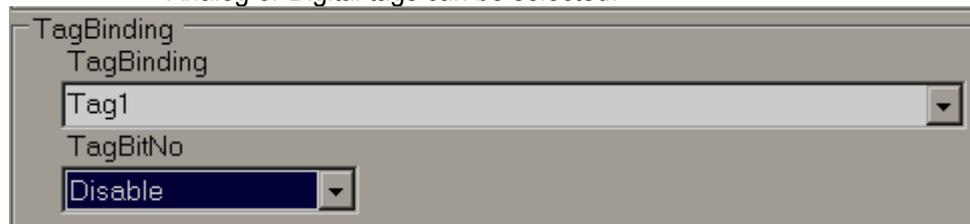
If Tag1 is an Analog Type (32 bit), it is also possible to show a different display based on individual bits. By default, it is disabled. You can select the bit from the combo box and then configure the band editor per project requirements.
