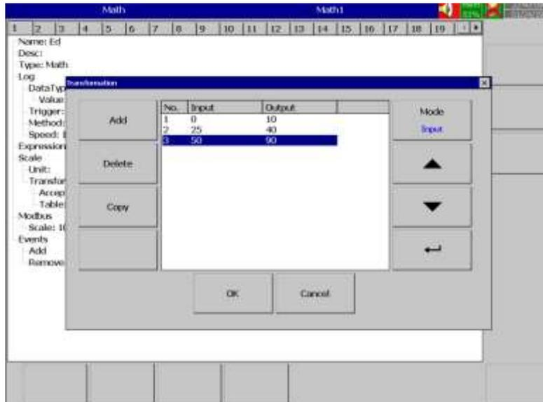
The high scale of this channel is 90 and the low scale of this channel is 10. The value of math channel is 68. The value at the Modbus register is 3092376452. The register value can be converted to math channel actual value by using the below conversion.
