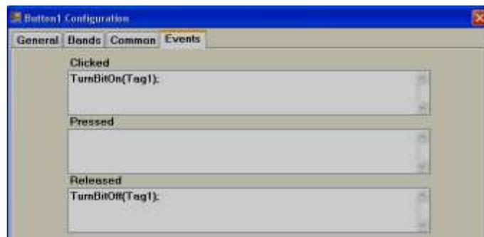
**Example:** Operator presses button for only 200msec. When the operator clicks the button, Tag1=1. When operator releases the button, Tag1 = 0, holding time = 1000 msec.
