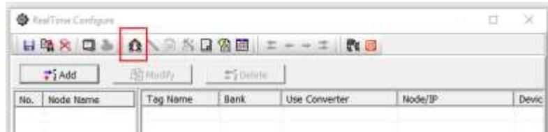
5. There are 4 different banks are available for the user to configure. It will allow the software to read the data from different communication networks like RS232, RS485, and Ethernet.
