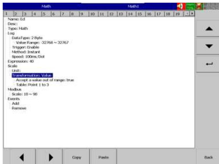
The scale low and scale hi of the math channel can be referenced from transformation table output values. For example, the transformation table configured as below.
