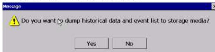
Press on “Yes” to dump data from internal memory to external SD Card or USB memory.
