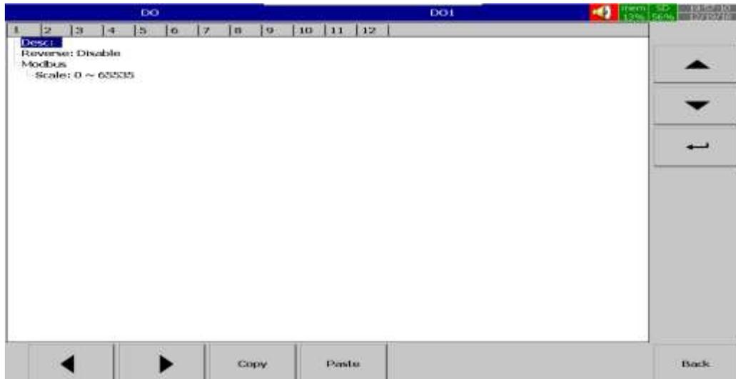
**Copy:** copy the channel configuration from one channel to another channel.
