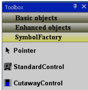
In Toolbox, click “Symbol Factory”, then drag and drop a standard control to the screen.
