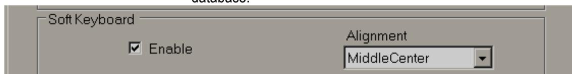
**Soft keyboard:** If enabled, it is possible to control the keypad appearance during run time. For example, if “alignment” is selected as the Middle centre, then, when the keypad appears during run time, it will be located in the middle-centre of the screen
