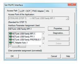
III. It is possible to adjust the station-related parameters in the properties of the NETLink® USB Family, if necessary. Otherwise the access path to the connected controllers is now defined with this setting, and it is possible to work with the Simatic¹ engineering programs.
