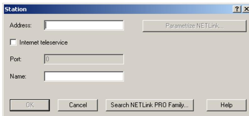
To able to access a NETLink® with the NETLink-S7-NET driver, a station must be set up first. This station is virtually and is not stored in the NETLink® Gateway hardware – it permits easier differentiation if several NETLink® devices from the NETLink® family are used.
