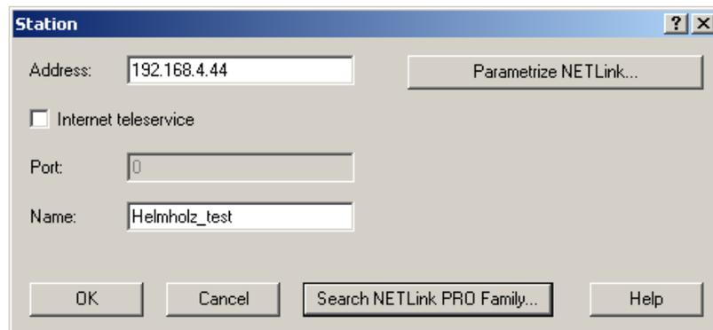
The 'Parameterize NETLink ...' button takes you to a new input form that already contains the current parameters of the NETLink®:
