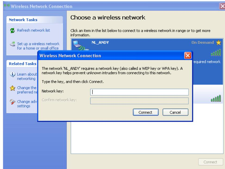
4. Step: Now enter the valid key for the respective NETLink® WLAN and confirm by clicking the 'Connect' button. Windows does not display the key, either, but keeps the characters hidden.
