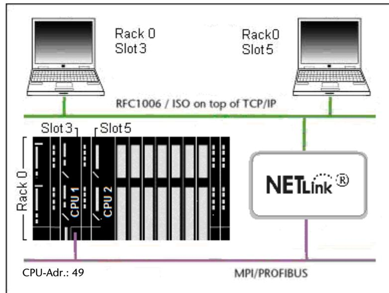
The rack/slot address for the station that will be used to communicate on the rack must be configured in the communication software (in the above example: R/S = 0/3 for CPU 1 and R/S = 0/5 for CPU 2)
