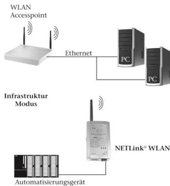
When using the infrastructure mode the communication of two WLAN components is handled by a mediation unit, an access point (AP). The AP functions as central coordination point of the
