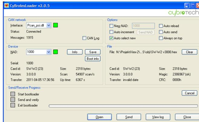
IEX modules have IEX bootloader, programmed in hardware programmer. Atmel bootloader is not supported. Bootloader is compatible with programs v3.x.x.x. IEX modules can be re-programmed in a running network, not affecting other modules. CyBro may also be connected and running. IEX Loader opens hex files only, binary files are not supported.
