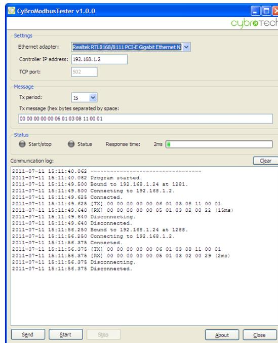
Tester is MODBUS/TCP master, tested device (CyBro) is MODBUS/TCP slave. Tester works in a local network, direct connection is not supported (i.e. CyBro should have valid IP address).
