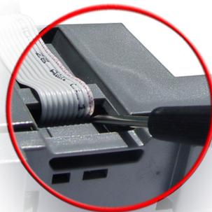
3. Gently remove the top of the device as shown.
