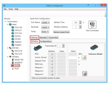
Ensure that the Port name, Baudrate, Parity and the Modbus Address fields are the same obtained in configuration mode.
