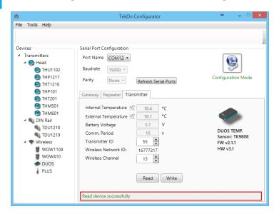
The device's identification data is now available in the software window. In this guide, the *DUOS TEMP Wireless Transmitter* has been considered.
