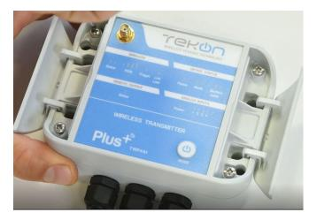
Connect a micro USB cable to the computer and then to TWP4AI PLUS Wireless Transmitter.
