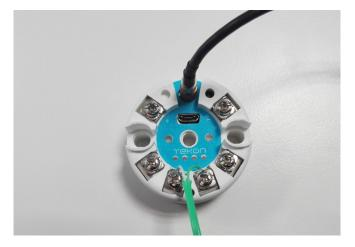
Connect the micro USB cable to the computer and then to TWPH-1UT PLUS Wireless
