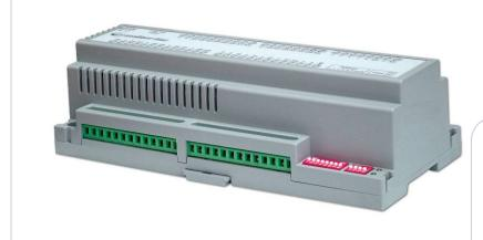
Main Controller for Fan Coil in Building Management System (B.M.S.) applications, with RS-485 interface to BACnet protocol and Pulse Modulating outputs for the Fan-Coil valves
