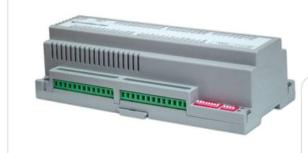
Main Controller for Fan Coil in Building Management System (B.M.S.) applications, with RS-485 interface to BACnet protocol and proportional (0-10V) outputs for the Fan-Coil valves
