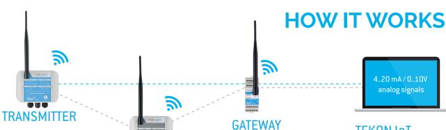
Featuring wireless mesh network technology performing up to 4 Km encrypted communication range, this device can turn any third-party sensor with an analog output into an IoT wireless smartsensor. PLUS Wireless Transmitter supports up to 4 configurable analog inputs (4..20 mA/0..10 V) for instantaneous cable replacement as well as digital inputs and outputs for basic remote interactions.
