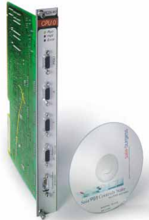
The 15-year old PCD6.Mxxx CPU series: upgradeable with Ethernet-TCP/IP and still programmable with the latest Saia® software tools
