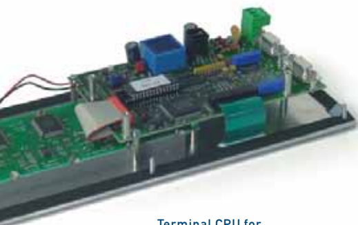
Terminal CPU for high-volume OEM with in-house control system
